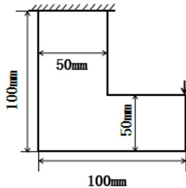
Figure 5. A loaded knee structure.
