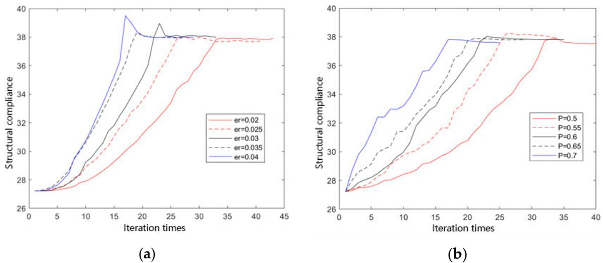
Figure 6. Evolution histories of structural mean compliance at different rates: (a) the changes in the structural compliance using different deletion rate; (b) the changes in the structural compliance using different minimum variation rate.
