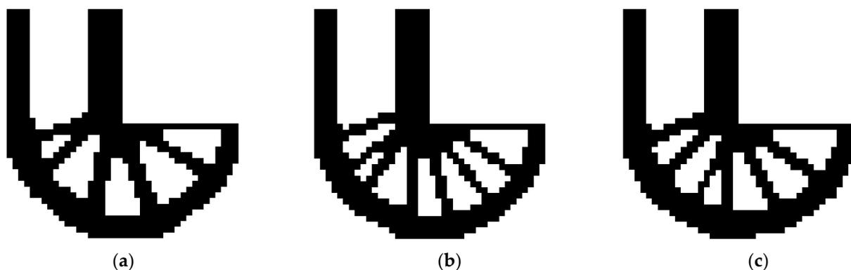
**Figure 8.** Topological configurations obtained by the two algorithms. (a)  $C = 37.8189$ ,  $t = 25$ . (b)  $C = 37.7605$ ,  $t = 27$ . (c)  $C = 37.9437$ ,  $t = 27$ .
