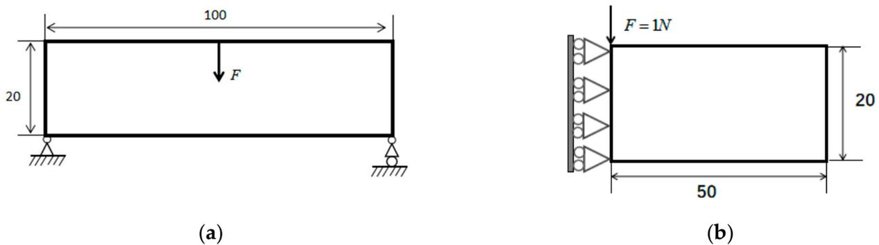
**Figure 2.** Design domain of a Michell-type structure: (a) two-dimensional simply supported beam; (b) the design area of the right half of the beam.
