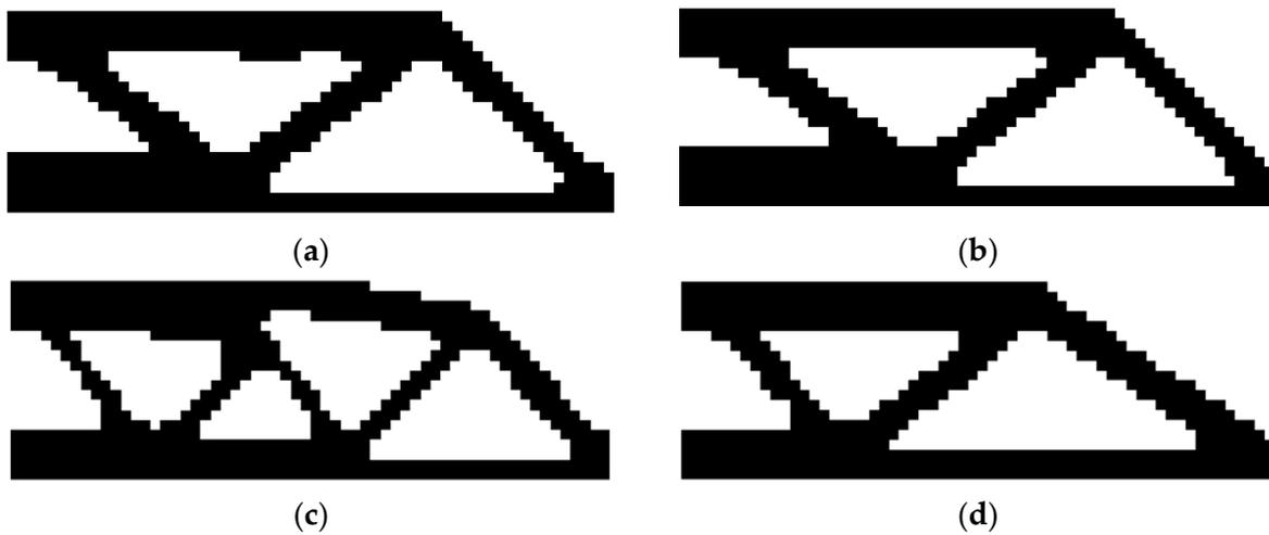
**Figure 3.** Optimal topology for the Michell-type structure. (a)  $C = 94.4720$ ,  $t = 63$ . (b)  $C = 95.6902$ ,  $t = 60$ . (c)  $C = 96.0235$ ,  $t = 57$ . (d)  $C = 96.6927$ ,  $t = 56$ .
