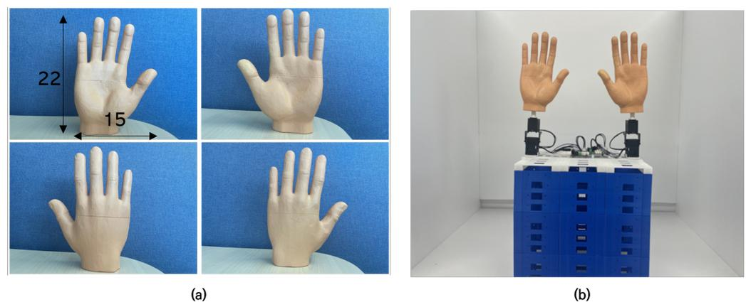
**Figure 7.** Our robot arm used for ground truth: (a) hands made by modeling, the unit is cm; (b) robot arms.
