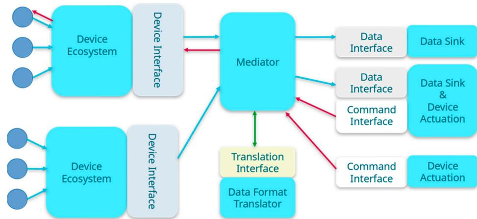
**Figure 1.** Generic architecture for CPS Framework.
