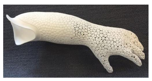
Figure 5. 3D printed prosthetic socket and arm produced using PBF.
