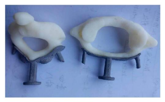
Figure 16. Fitting of the metal template to the FDM-printed cervical vertebra model [108].
