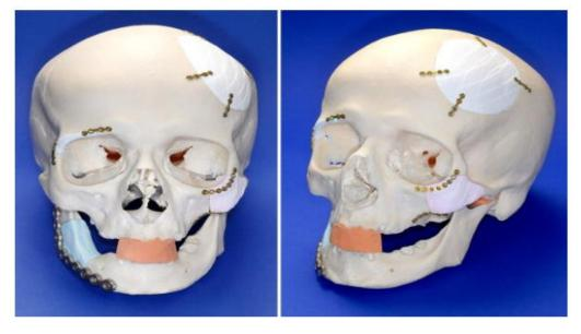
Figure 10. Skull with 3D-printed embedded implants [86].
