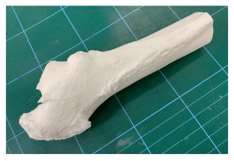
Figure 9. Bone-drilling practice part made with powder bed fusion.
