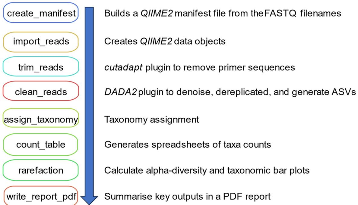
**Figure 1.** A summary of the *Snakemake* rules used to execute the *eDNA-container app* pipeline. Each box represents a *Snakemake* rule that runs a specific step in the pipeline as indicated by the description. The rules are executed in the order indicated by the arrow.
