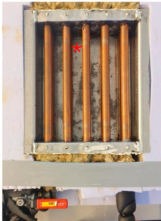
Figure 4. Picture of the shell-and-tube TES tank (“\*” represents the position of the thermocouple).
