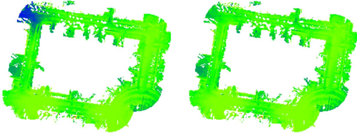
**Figure 9.** Point cloud deformation by inaccurate determination of the control point.
