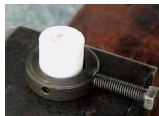
Figure 7. Sample clamping during CMM measurements.
