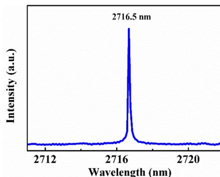
**Figure 7.** Spectrum of the Q-switched Er:Y<sub>2</sub>O<sub>3</sub> laser.
