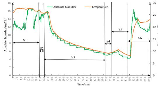
Figure 6. The absolute humidity and temperature fluctuation in the fresh fruit cold chain.
