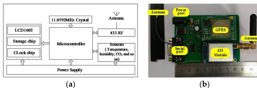
**Figure 2.** The physical implementation of the WSN (wireless sensor network) nodes. (a) The flow chart of slave sensor node; (b) Hardware of master sensor node.
