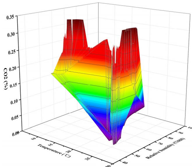
Figure 7. The CO<sub>2</sub> level change with temperature and relative humidity fluctuation for the peach and nectarine cold chain.
