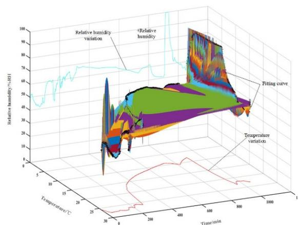
Figure 5. The relative humidity and temperature fluctuation in the fresh fruit cold chain.
