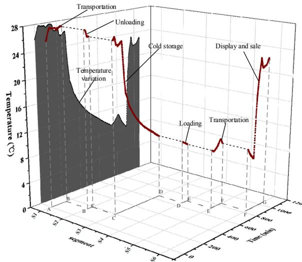
Figure 4. The temperature fluctuation in the fresh peach and nectarine cold chain.
