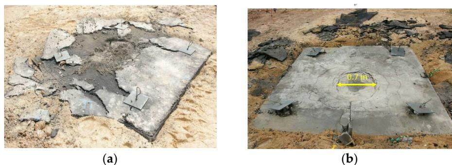
**Figure 11.** Damage of the multi-layer pavement after blast loading: (a) damage pattern of the AC layer in field blast test; (b) damage pattern of the HSC layer in field blast test.
