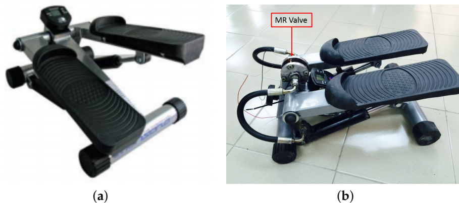
Figure 1. Conventional Stepper vs Modified stepper. (a) Conventional stepper; (b) Modified stepper (magnetorheological (MR) valve).
