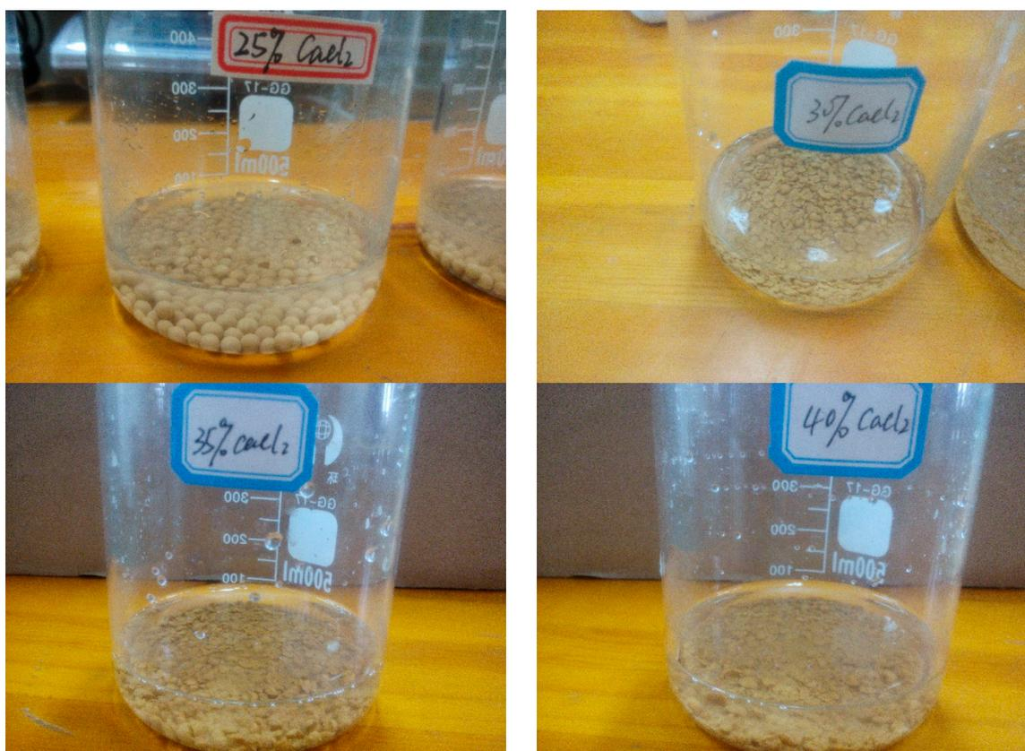
Figure 1. 13X/CaCl<sub>2</sub> composite adsorbent.
