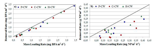
**Figure 3.** Endocrine disruptive compound(EDC) removal rate for H-CW, C-CW, and P-CW against their mass loading rates (**a**) BPA and (**b**) NP. Continuous line represents 100% removal.
