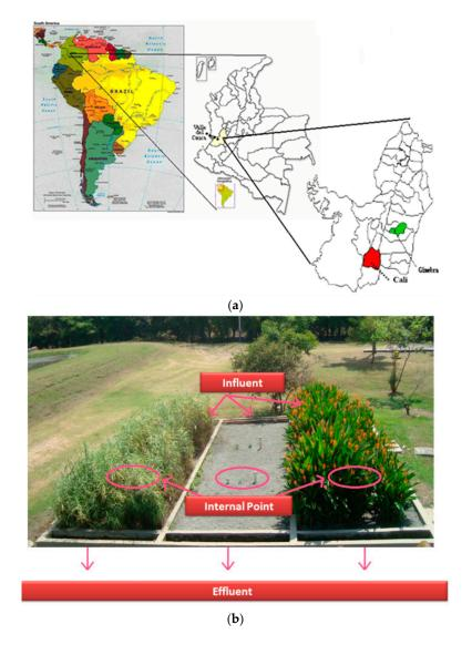
**Figure 1.** (a) Location of the pilot scale; (b) pilot scale horizontal subsurface flow constructed wetlands used in this study.
