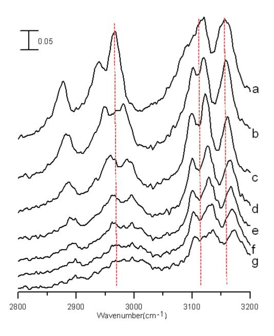
**Figure S1.** IR spectra of the mixture after 2 washes with ethanol obtained under ambient pressure (curve a) and at 0.4 (curve b), 0.7 (curve c), 1.1 (curve d), 1.5 (curve e), 1.8 (curve f), and 2.5 GPa (curve g).
