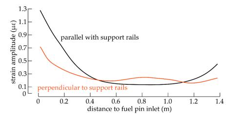
**Figure 7.** The trend of the rms vibration amplitude (in terms of strain) measured with the different FBGs located on the central fuel pin in the two perpendicular directions with respect to the support rails.
