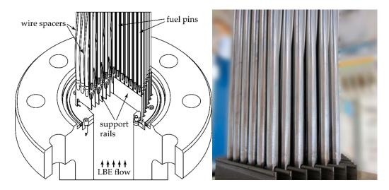
Figure 3. Concept drawing and photograph of the fuel assembly inlet.
