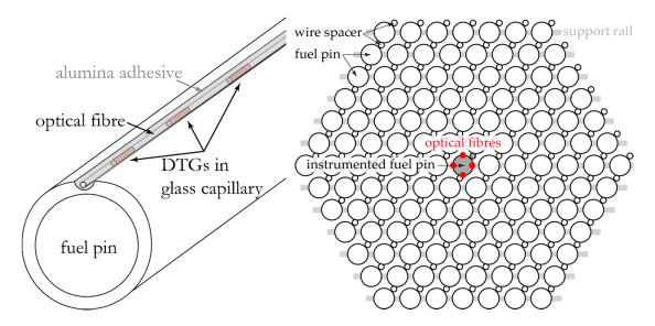
**Figure 4.** (Left) Scheme of an optical fibre with draw tower gratings (DTGs) embedded in a small groove on the surface of the pin. (**Right**) The location of the instrumented fuel pin with 4 fibres (represented by the red dots) containing in total 84 FBGs.
