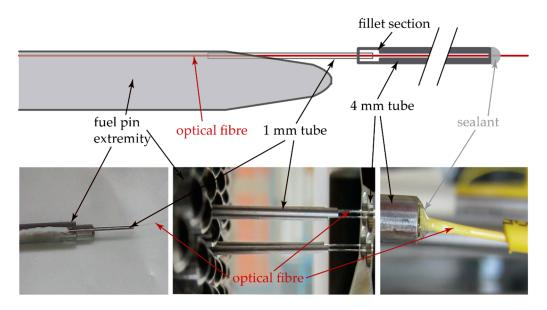
**Figure 5.** Illustration of the alignment set-up designed to avoid affecting the vibration due to the egress of the optical fibre and its guide capillary. Note that for sake of readability, the figure is not to scale.
