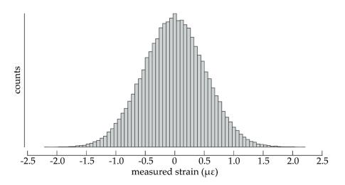
**Figure 8.** The histogram of the vibration (in terms of strain) gives a more complete view of the fuel pin vibration. Average strain amplitude exceeding 2 με rarely occurs at MYRRHA nominal flow speeds.
