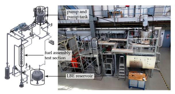
**Figure 2.** (Left) Isometric view of the experimental test facility in which the flow induced vibrations of a full-scale lead-bismuth eutectic (LBE) cooled fuel assembly were tested. (**Right**) A photograph of part of the facility above ground-level.
