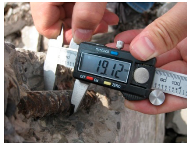
Figure 2. Cover depths measurement.
