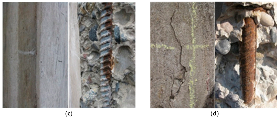
Figure 5. States of columns before and after breaking: (a) uncracked with uncorroded (Sample C2); (b) uncracked with minor corrosion (Sample B6); (c) uncracked with moderate corrosion (Sample A22); (d) cracked with severe corrosion (Sample C1).
