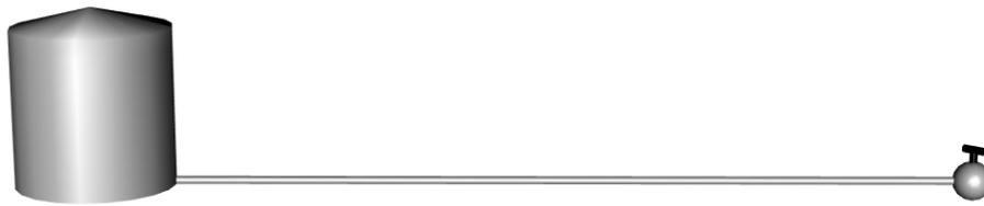
**Figure 2.** Reservoir-pipe-valve system with a straight pipe which is free to move in the axial direction.
