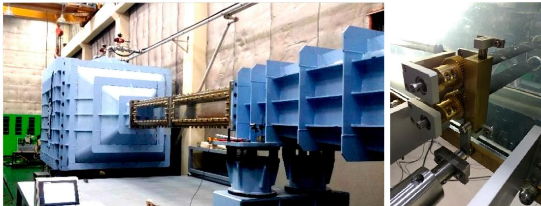
Figure 18. Experimental set-up: (a) high-speed cavitation tunnel; (b) gust generators with driving devices.
