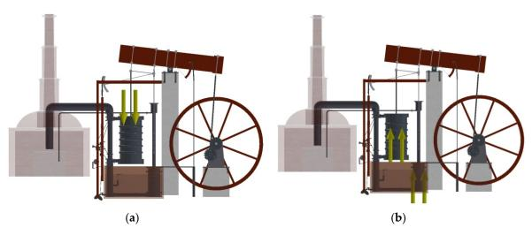
Figure 8. Force transmitted by the piston: (a) downward movement and (b) upward movement.
