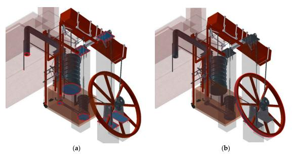
**Figure 5.** Embedded supports: (**a**) fixed elements (**b**) inertia flywheel defined as a built-in element to simulate stop situation.
