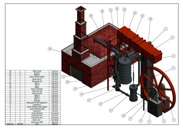
Figure 1. Isometric view of the double-acting steam engine.
