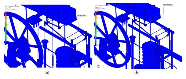
**Figure 16.** Location of the second highest von Mises stress: (a) downward movement and (b) upward movement.
