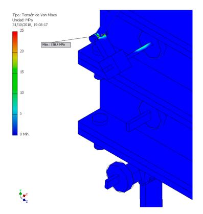
Figure 15. Location of the point where the von Mises stress is maximum.
