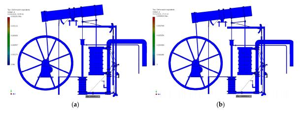
Figure 20. Equivalent deformations: (a) downward movement and (b) upward movement.
