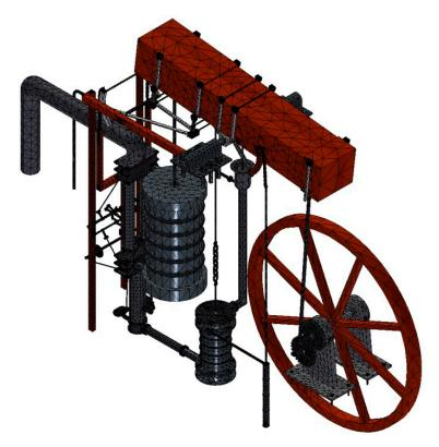
Figure 11. Automatic mesh obtained from the double-acting steam engine.
