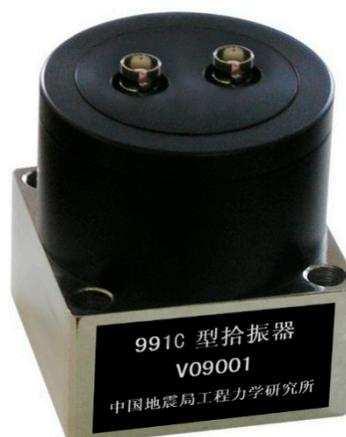
Figure 14. Model 991C accelerometer.
