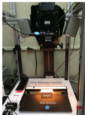
**Figure 2.** Hyperspectral imaging setup.
