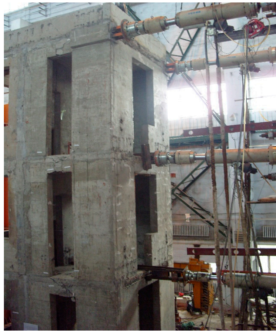
Figure 4. Arrangement of horizontal loading devices.
