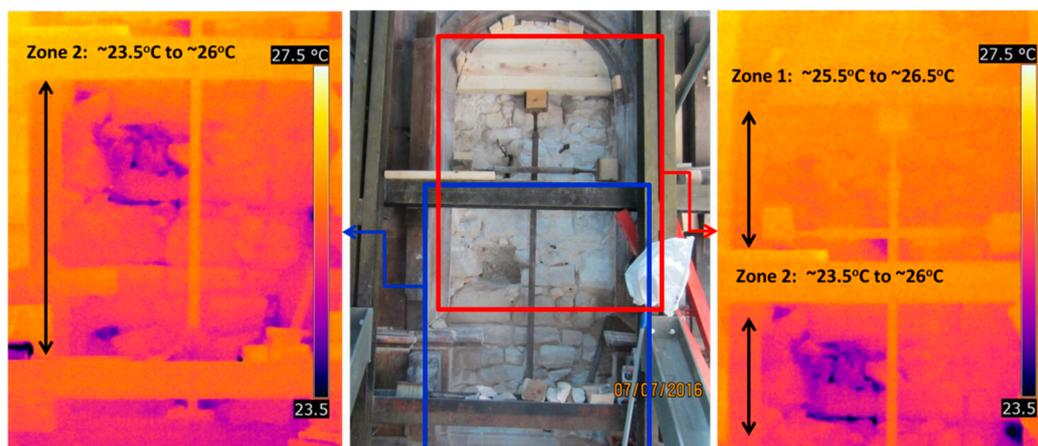
Figure 37. N2 panel masonry after filling mortar removal and respective IRT measurements.
