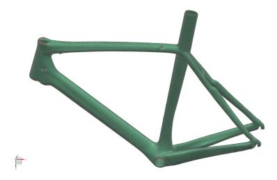
Figure 3. Overview of the 2D mesh of the bicycle frame.
