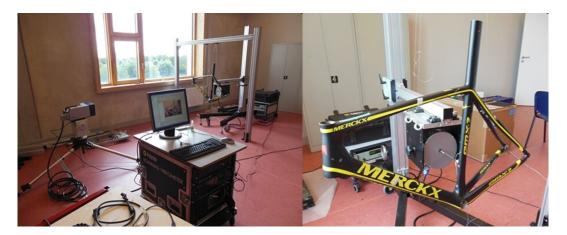
Figure 2. Photograph of the modal analysis measurement setup.
