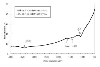
Figure 2. FTIR spectrum of TPCB.
