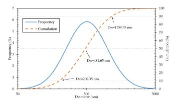
Figure 3. The Gaussian fit of laser size analysis of TPCB.
