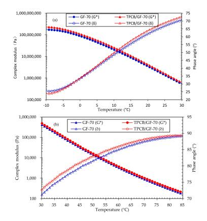
**Figure 5.** G\* and  $\delta$  of GF-70 and TPCB/GF-70 in the temperature range of  $-10 \sim 30 \circ \text{C}$  (a) and  $30 \sim 85 \circ \text{C}$  (b).
