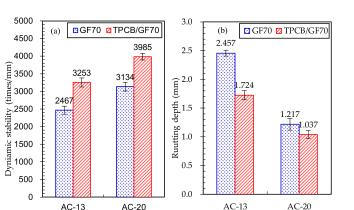
Figure 8. DS (a) and rutting deeps (b) of GF70 and TPCB/GF70 asphalt mixtures.
