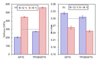
Figure 7. Stiffness (a) and m-value (b) of GF-70 and TPCB/GF-70.
