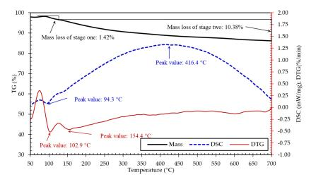
Figure 4. TG, DTG, and DSC curves of TPCB in the temperature range of 50 °C to 700 °C.
