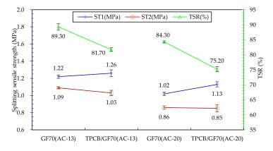
Figure 11. Results of freeze-thaw splitting testing of GF70 and TPCB/GF70 asphalt mixtures.
