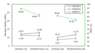
Figure 10. Results of immersion Marshall testing of GF70 and TPCB/GF70 asphalt mixtures.
