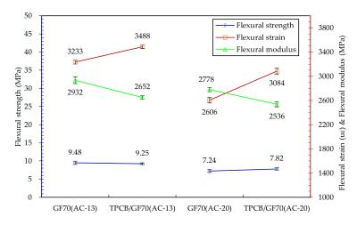
Figure 9. Results of low-temperature bending test of GF70 and TPCB/GF70 asphalt mixtures.
