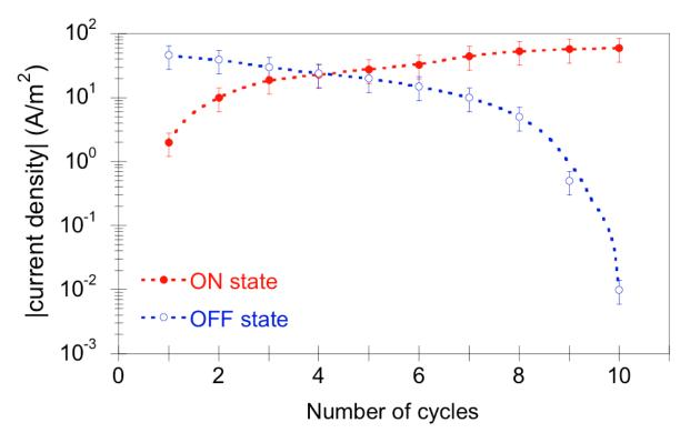
**Figure S3.** Variation of the current density (in ON and OFF state) versus the number of sweeping voltage cycles. The current density was measured for an applied voltage of +/-5 V.
