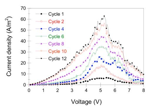
**Figure S1.** indicated the evolution of NDR peak after several positive sweeping cycles (from 0 to +14 V). Positive poling procedure consists in performing several sweeping voltage cycles from 0 to +14 V, till the intensity of the current peak tends to saturate.
