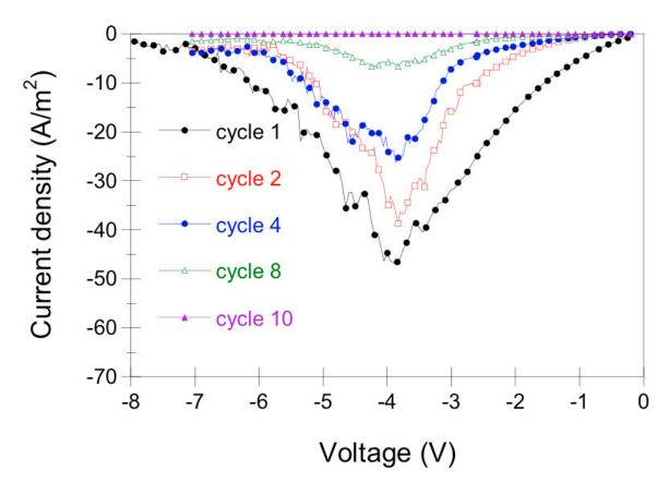
**Figure S2.** Evolution of NDR peak after several negative sweeping cycles (from 0 to -14 V). Negative poling procedure consists in performing several sweeping voltage cycles from 0 to -14 V, till the intensity of the current peak is lower than  $10 \text{ mA/m}^2$ .
