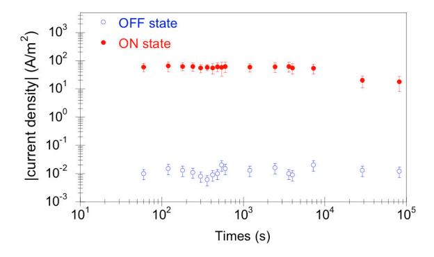
**Figure S4.** Retention time of both ON and OFF states measured at room temperature by applying constant voltage of 5 V. The current densities of both states (JoN and JoFF) do not show significant degradation after  $10^4$  s.
