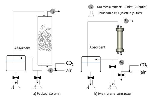
Figure 1. Experimental set ups for CO<sub>2</sub> capture.
