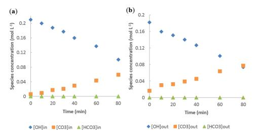
**Figure 3.** Evolution of inlet (**a**) and outlet (**b**) species concentration as a function of time in the membrane contactor.  $CO_2$  and NaOH initial concentrations are 10% and 0.2 mol L<sup>-1</sup>, respectively; gas and liquid flow rates are 6.5 and 1 L min<sup>-1</sup>; respectively.
