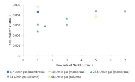
**Figure 4.** Mass transfer coefficient in function of the NaOH flow rate for different flue gas flow rates in the two set ups. The CO<sub>2</sub> and NaOH initial concentrations are 10% and 0.2 mol L<sup>-1</sup>, respectively, for all the cases except the experimental point corresponding to 23.7 L min<sup>-1</sup> gas (membrane) and 3 L min<sup>-1</sup> of NaOH flowrate, where it was used as 15% of CO<sub>2</sub>.
