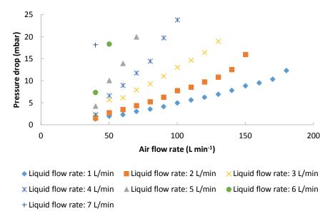
Figure A1. Pressure drop as a function of the air flow rate for different liquid flow rates.
