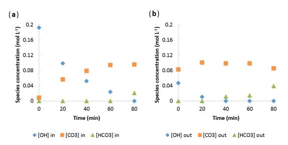
**Figure 2.** Evolution of inlet (**a**) and outlet (**b**) species concentration as a function of time in the packed column.  $CO_2$  and NaOH initial concentrations are 10% and 0.2 mol L<sup>-1</sup>, respectively; gas and liquid flow rates are 33 and 1 L min<sup>-1</sup>; respectively.
