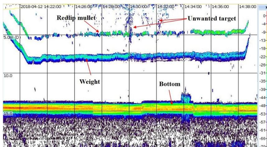
**Figure 3.** A sample echogram of the Redlip mullet ( $FL$ : 35.0 cm) from the *ex situ* target strength measurements.
