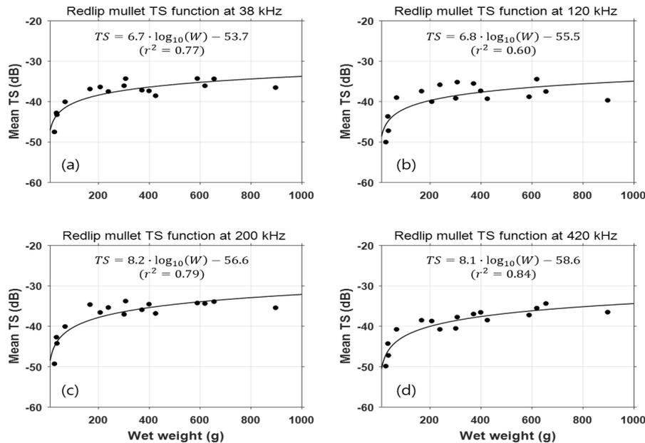
**Figure 6.** Relationship between the target strength (*TS*) and wet weight (*W*) at (a) 38, (b) 120, (c) 200, and (d) 420 kHz. Points represent the mean *TS* values, and solid lines represent least-squares regressions of mean *TS*.
