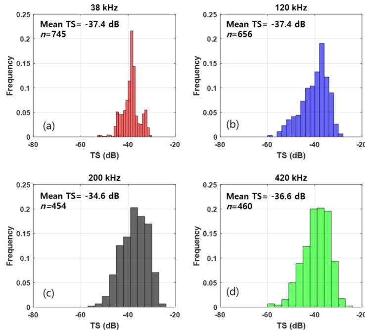
**Figure 4.** Representative target strength (*TS*) histograms of mullet (*FL*: 35.0 cm) at (a) 38, (b) 120, (c) 200, and (d) 420 kHz. Index, *n* is the sample size.
