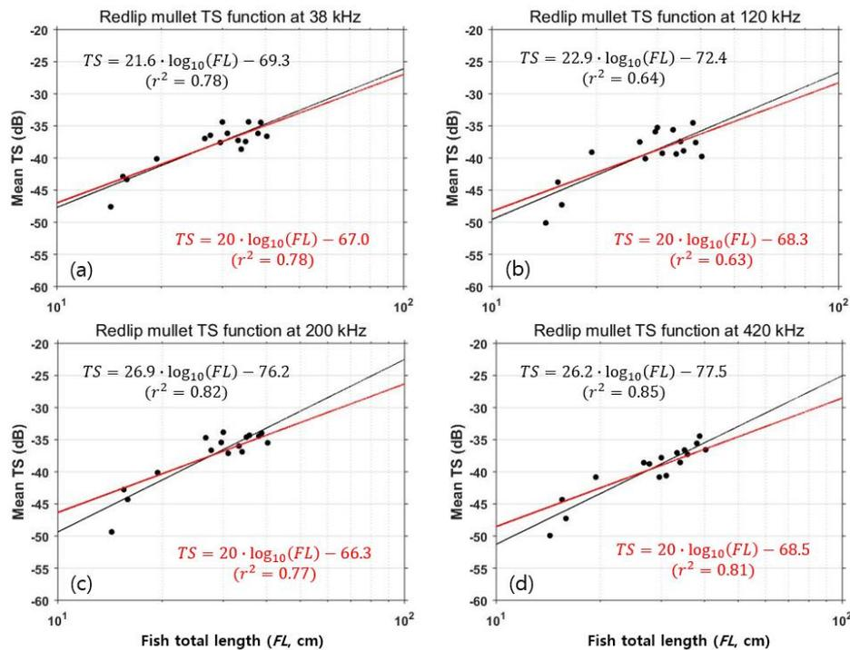
**Figure 5.** Relationships between target strength ( $TS$ ) and total fish length ( $FL$ ) at (a) 38, (b) 120, (c) 200, and (d) 420 kHz. Black points represent the mean  $TS$  values with  $FL$ . Black solid lines represent the least-squares regressions of mean  $TS$ , and the red solid line represents the standard fits of the  $TS$  functions.
