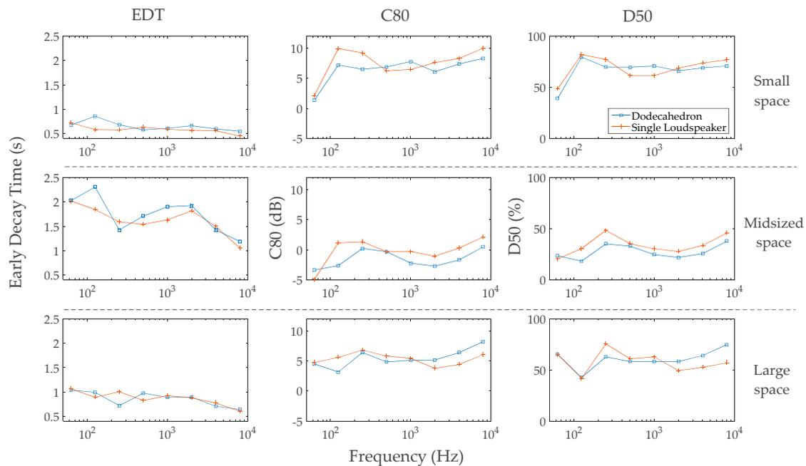
Figure 7. Early Decay Time (EDT), Clarity ( $C_{80}$ ) and Definition ( $D_{50}$ ) for the small, mid-sized and large space.
