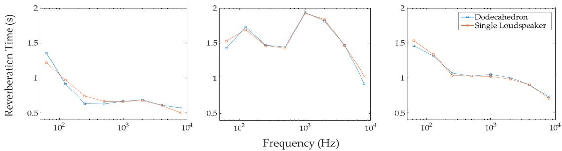
Figure 6. Reverberation Time (RT) for the small, mid-sized and large space (from left to right).
