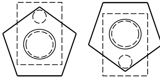
**Figure 3.** Placement of the face of the directional loudspeaker according to the placement of the face of the dodecahedron speaker (twelve positions measurements).
