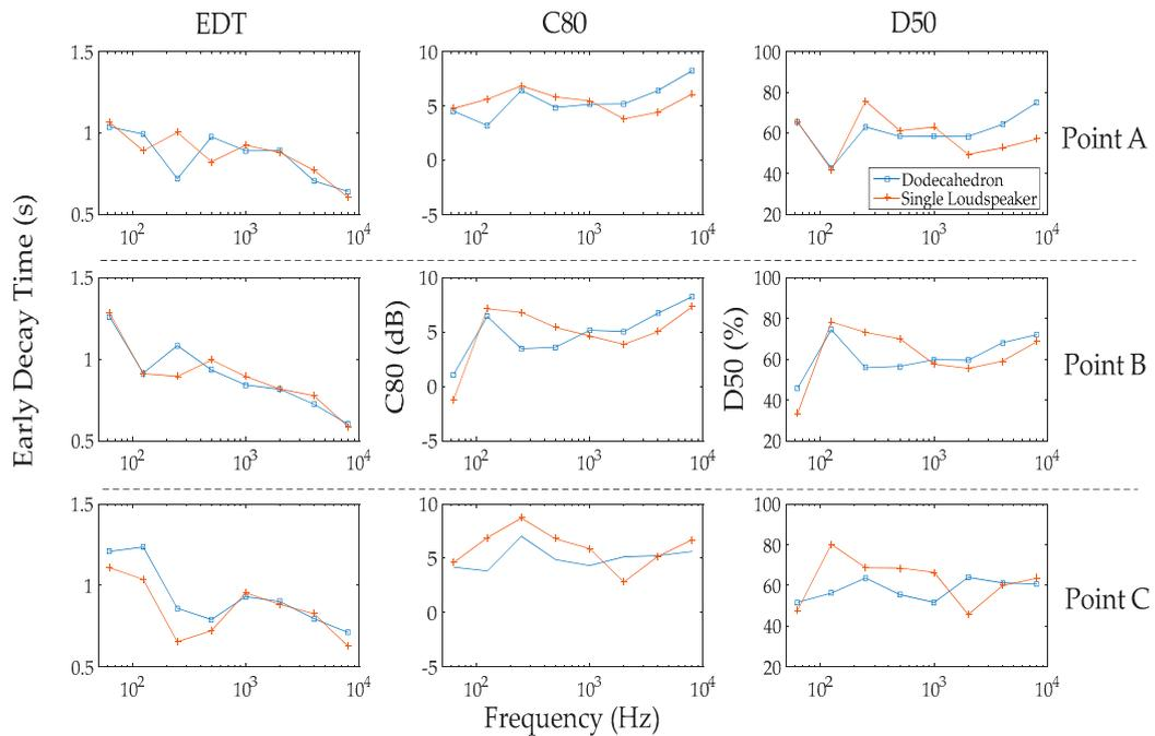
Figure 9. EDT,  $C_{80}$  and  $D_{50}$  for points A, B and C in the amphitheater.
