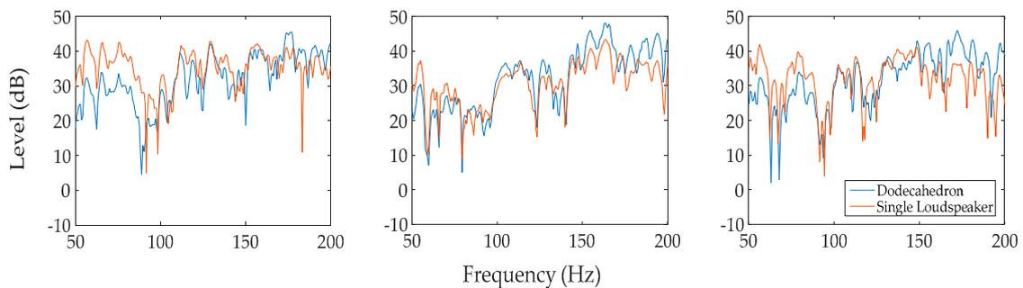
Figure 10. Frequency responses for measurements with the dodecahedron speaker and the proposed method for point A, B and C in the amphitheater (from left to right respectively).
