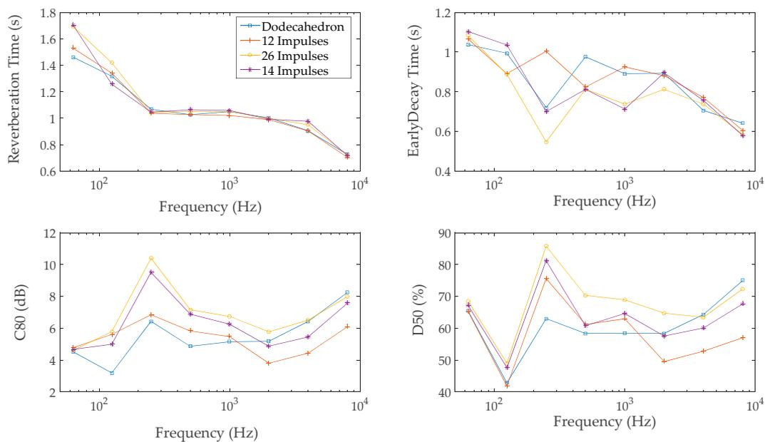
**Figure 11.** RT, EDT,  $C_{80}$  and  $D_{50}$  measured with different speaker placement methods.
