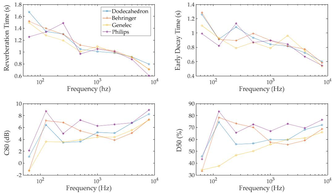
**Figure 12.** RT, EDT,  $C_{80}$  and  $D_{50}$  measured with different speakers.
