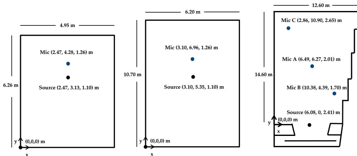
**Figure 1.** Source and microphone positions for the three spaces with volumes of  $88 \text{ m}^3$ ,  $192.4 \text{ m}^3$  and  $1088 \text{ m}^3$  (from left to right) where measurements were performed.
