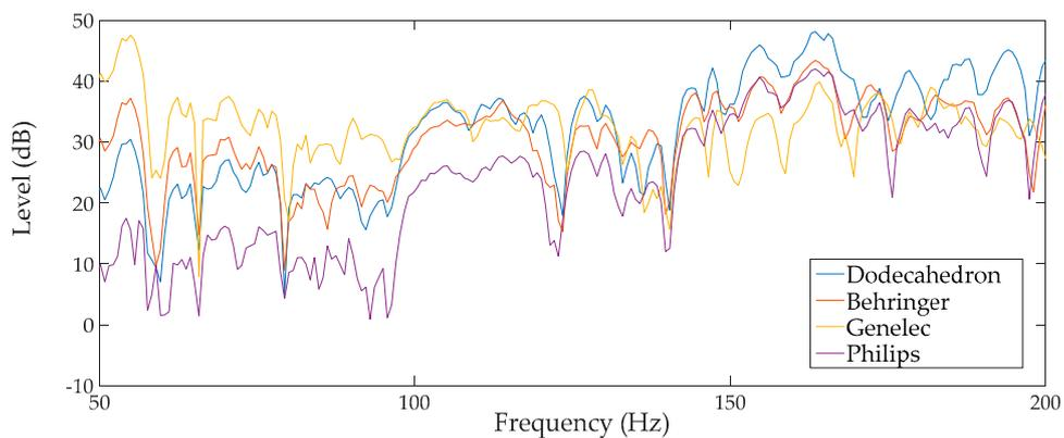
**Figure 13.** Frequency responses for measurements with the dodecahedron speaker and the proposed method with different speakers.
