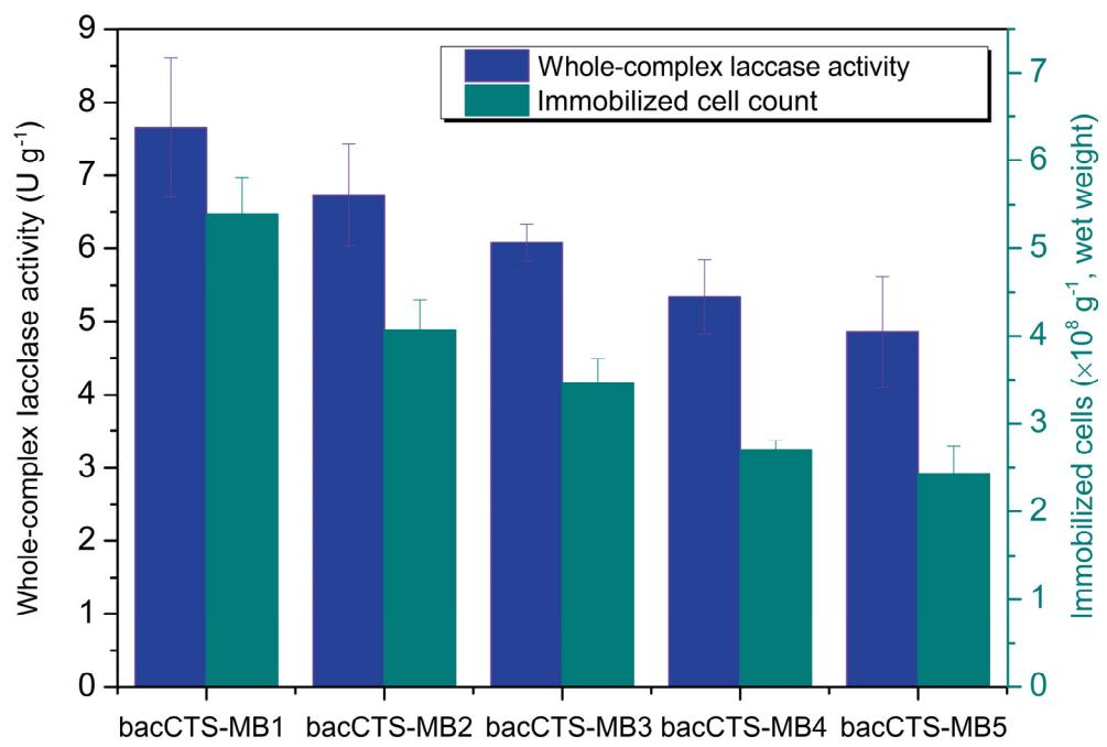
**Figure S4.** Whole-composite laccase enzyme activity and immobilized *P. putida* cell counts of the five prepared bacCTS-MB materials.
