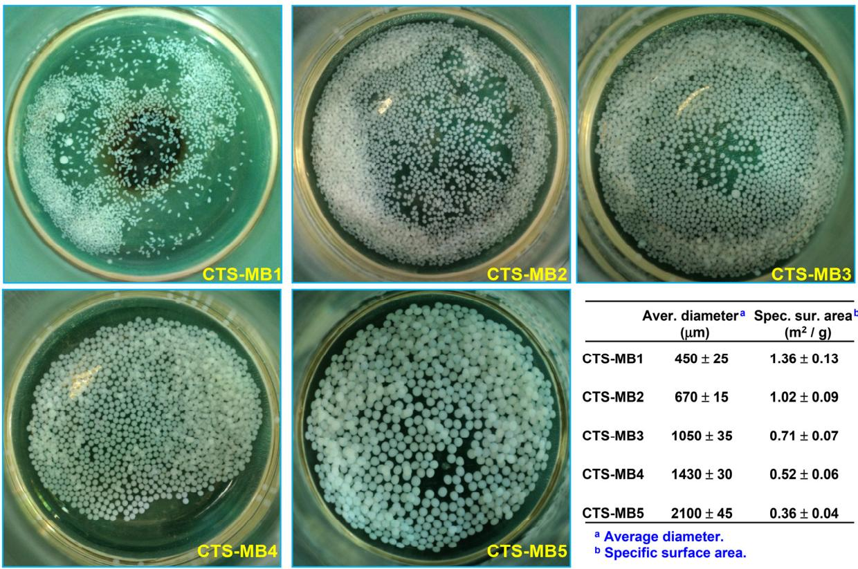
**Figure S3.** Morphological images of the five as-prepared CTS-MB materials and their average diameters and specific surface area values.
