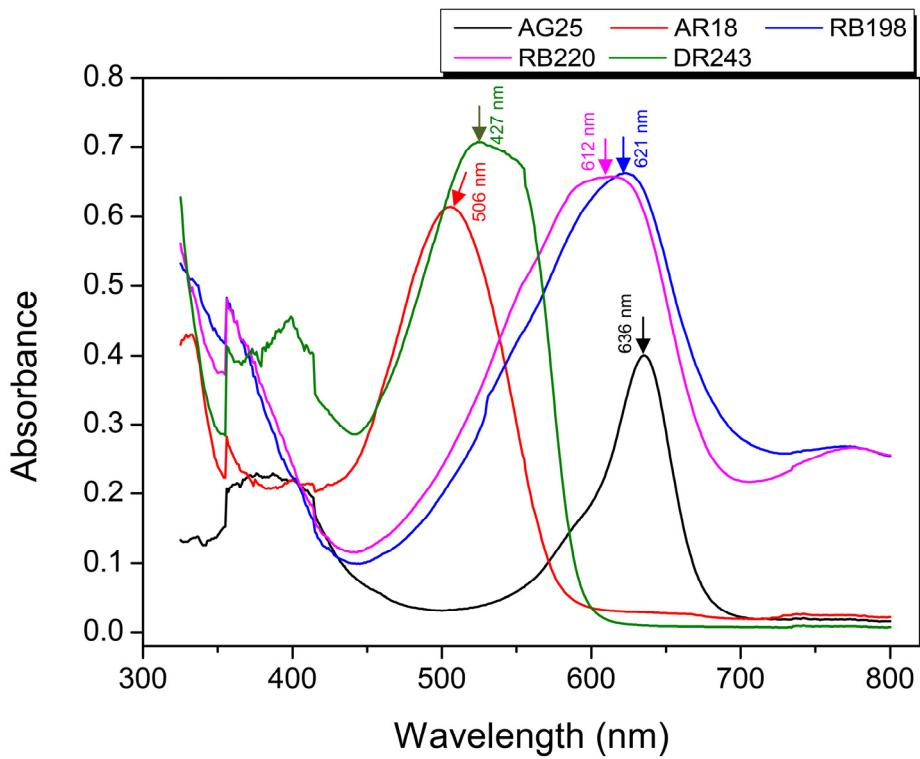
**Figure S2.** Full wavelength (325 nm to 800 nm) scanning curves of five synthesized dyes indicating their maximal adsorbent peaks (arrows), which were used as the OD values for the dye absorbance measurements.
