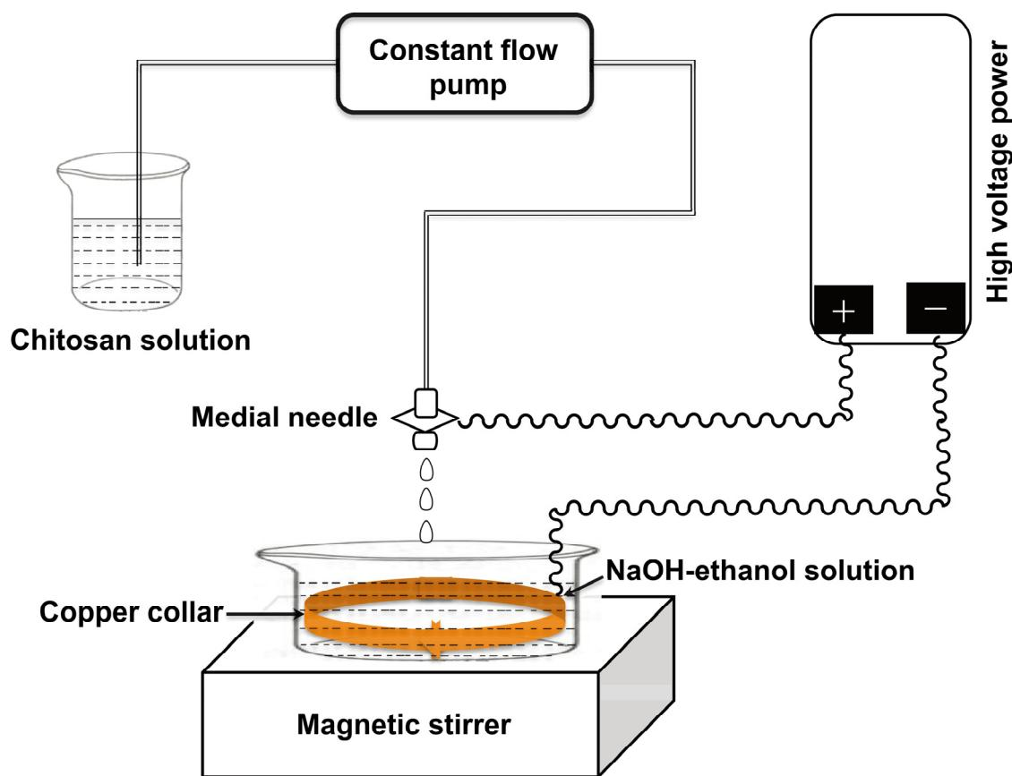
**Figure S1.** Schematic illustration of the self-assembled facile device for the preparation of various chitosan microbeads with different particle sizes.
