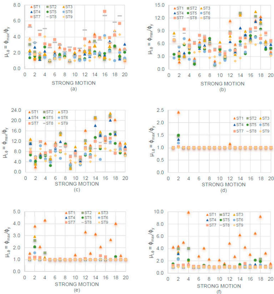
**Figure 4.** Bending local ductility ( $\mu_{L\phi}$ ), EW direction, 10-level building; beams: (a)  $S_a = 0.2$  g, (b)  $S_a = 0.6$  g, (c)  $S_a = 0.8$  g; columns: (d)  $S_a = 0.2$  g, (e)  $S_a = 0.6$  g, (f)  $S_a = 0.8$  g.
