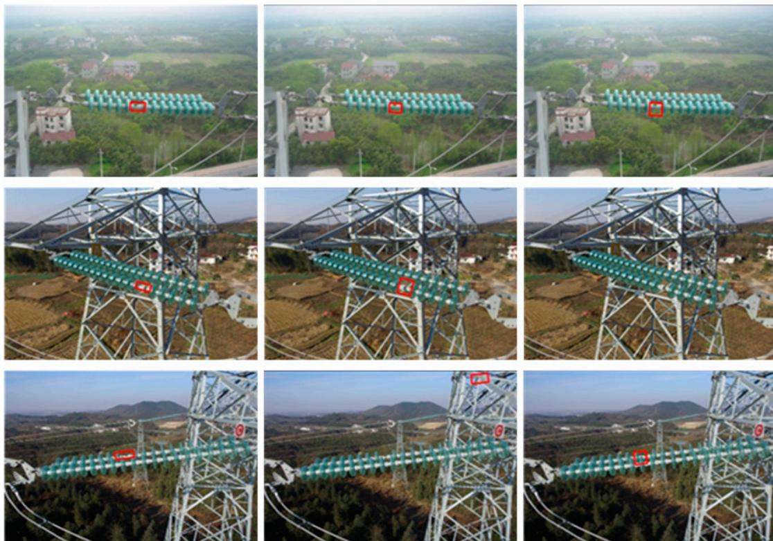
**Figure 9.** Experimental results in aerial images with insulator one fault. In each row, the first column to the third column depicts the performance of the proposed method, method [20], and method [11], respectively.
