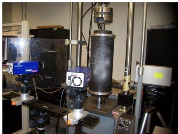
Figure 1. Axial buckling test setup for evaluating DIC [15].
