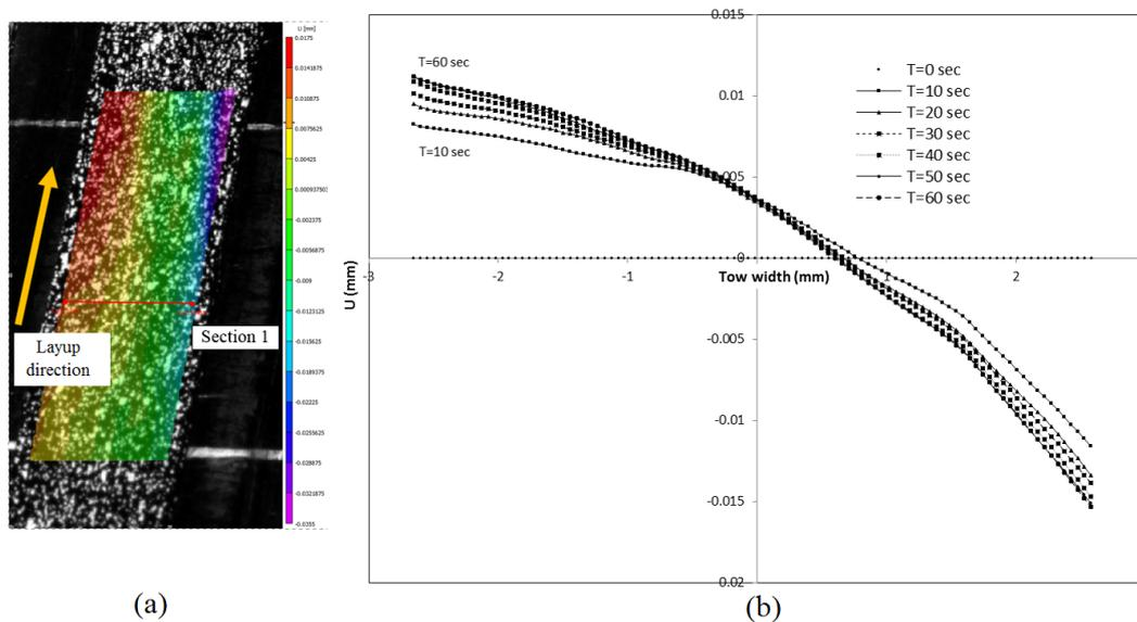
**Figure 19.** (a) Distribution of the lateral deformation along the width and length of the composite tow one minute after layup. (b) Variation of lateral deformation along the width of the composite tow one minute after layup [19].
