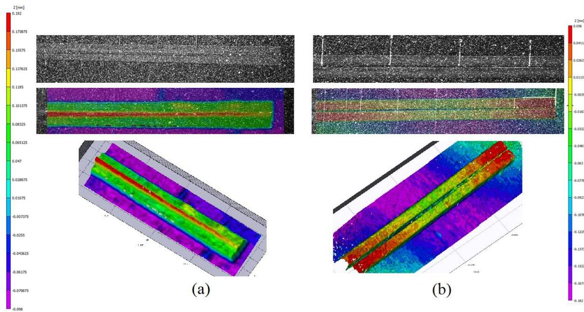
Figure 22. (a) Overlap between two tow detections. (b) Gap detection, z-axis represents thickness direction.
