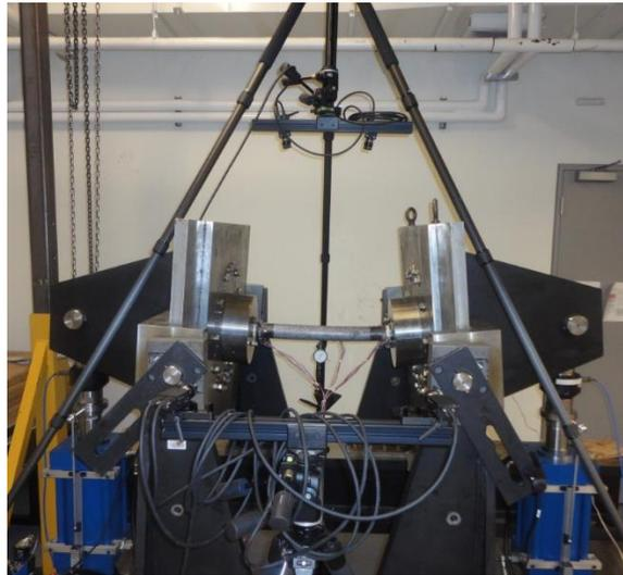
**Figure 12.** Bending test setup including the DIC system and thick composite tube (after failure) [16].
