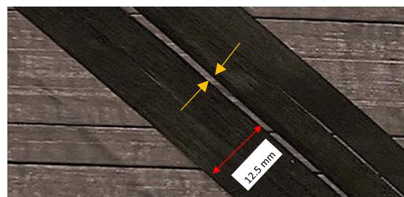
**Figure 20.** Gap size defect.
