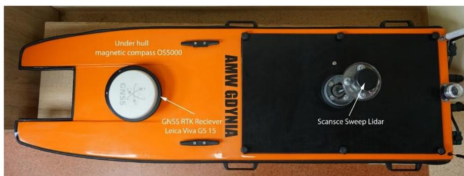
Figure 10. The distribution of measuring instruments on the unmanned surface vehicle (USV).
