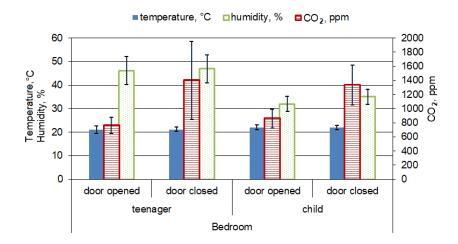
**Figure 3.** Mean temperature, relative air humidity, and CO<sub>2</sub> concentration inside the teenager's and child's bedrooms during the night.
