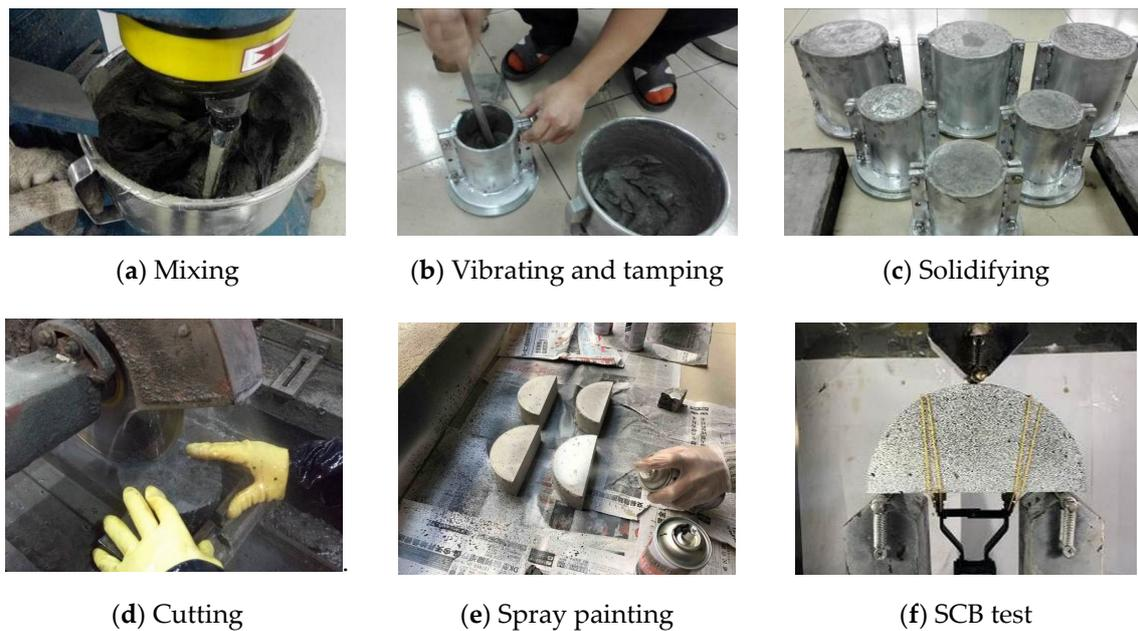
**Figure 3.** ECC semi-circular bending (SCB) specimen preparation process.
