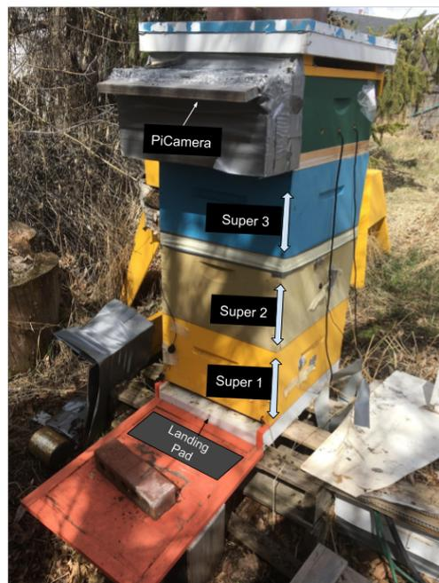
**Figure 1.** A BeePi monitor box on top of a Langstroth beehive that consists of 3 supers; the camera is protected against the elements with a specially constructed wooden box. More hardware details are available at [42,43].
