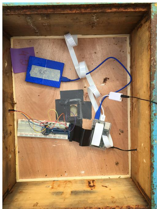
**Figure 2.** A BeePi monitor consists of a raspberry pi 3 model B v1.2 computer, a pi T-Cobbler, a breadboard, a waterproof DS18B20 temperature sensor, a pi v2 8-megapixel camera board, a v2.1 ChronoDot clock, and a Neewer 3.5 mm mini laval microphone placed above the landing pad. More hardware details are available at [42,43].
