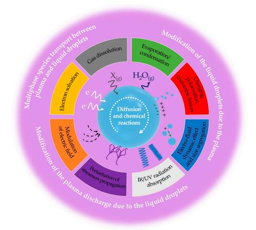
Figure 1. Schematic representation of the interactions between the plasma and an aerosol droplet.
