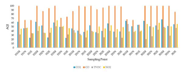
**Figure 9.** Indoor AQI for  $CO_2$ , CO, VOC, and  $NO_2$  for 27 sampling points. (The sampling name format is as follows: the first number indicates the Co-Op number, S is the spot location, M = morning, N = noon, and E = evening; for example, 2S3M = Co-Op 2, Spot 3, morning).
