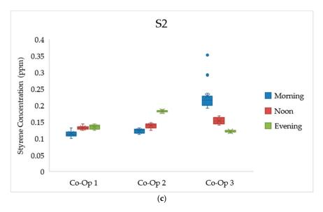
**Figure 6.** The volatile organic compounds concentration: (a) TVOCs in spot S3; (b) benzene in spot S1; (c) styrene in spot S2.
