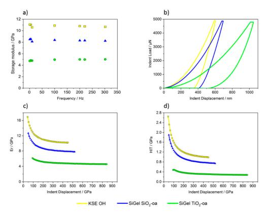
**Figure 1.** Mechanical properties of the xerogel on a microscale level. (**a**) Variation of the storage modulus with the sweep frequency; (**b**) load-displacement curves; (**c**) Dependence of Young's modulus (**c**) and hardness (**d**) on indent displacement.
