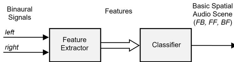
**Figure 1.** Block diagram of the basic spatial audio scene classifier (output categories are explained in the text). *FB*: foreground–background; *BF*: background–foreground; *FF*: foreground–foreground.
