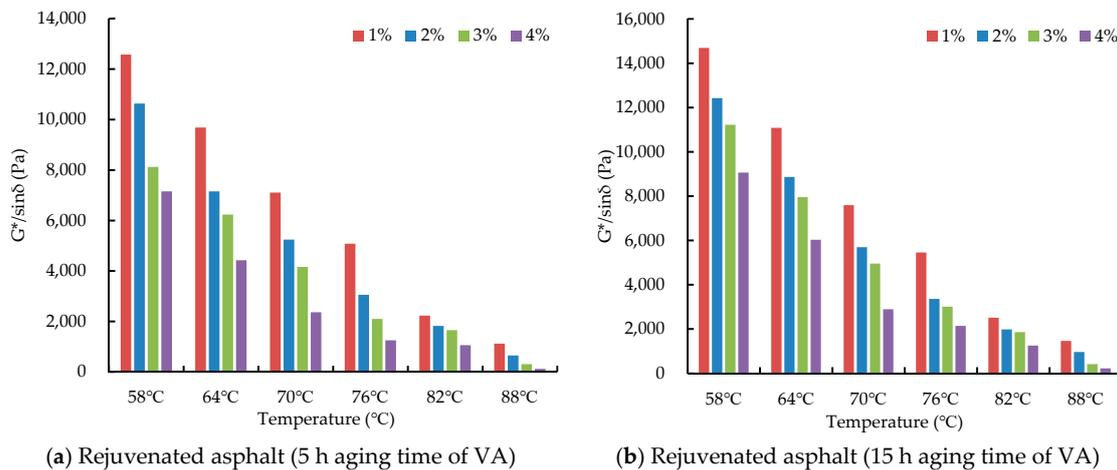
Figure 15. Influences of WEO on rutting resistance factor of rejuvenated asphalt (different aging time of VA).
