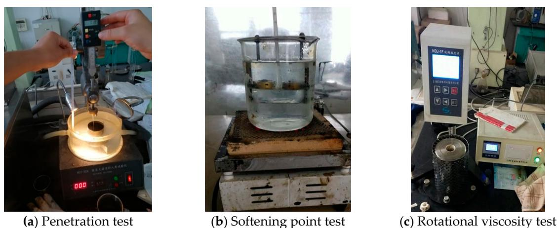
**Figure 4.** Basic physical properties tests of rejuvenated asphalt with WEO or WCO.
