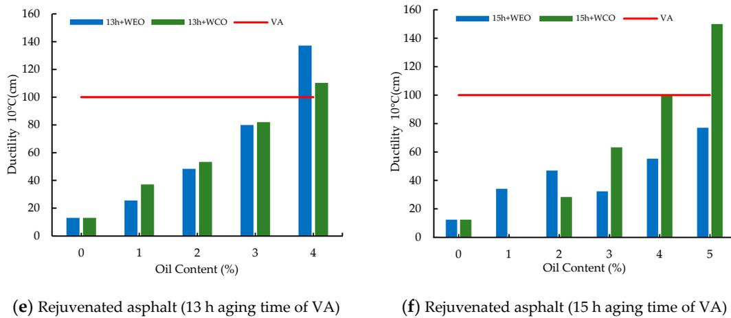
**Figure 8.** Effects of WEO and WCO on ductility of different aged asphalts at 10 °C.
