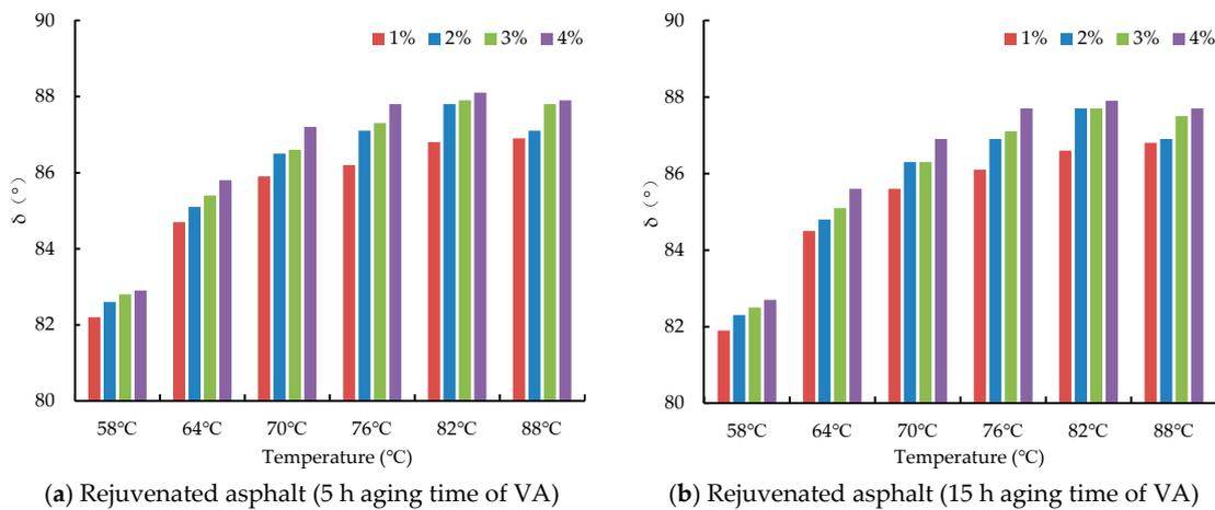
Figure 12. Influences of WCO on phase angle of rejuvenated asphalt (different aging time of VA).
