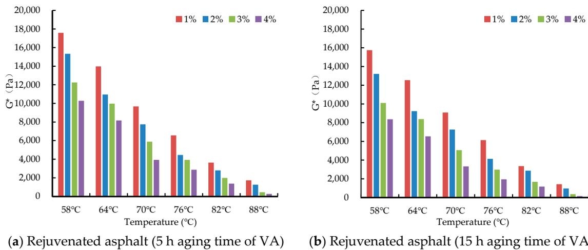
Figure 13. Effects of WEO on complex modulus of rejuvenated asphalt (different aging time of VA).
