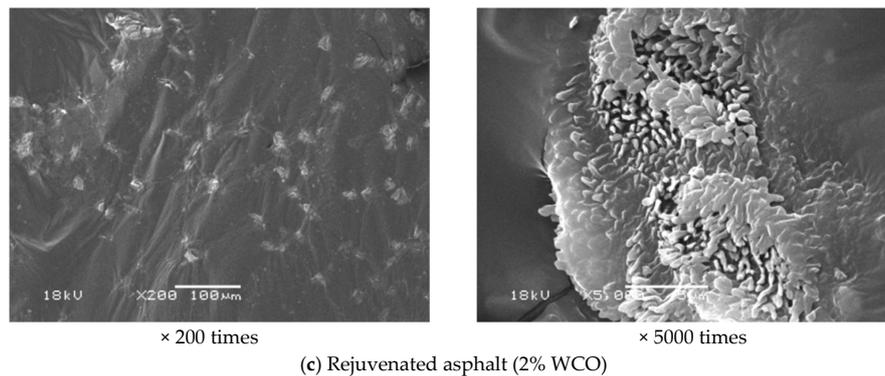
**Figure 18.** The SEM images of different asphalt states.
