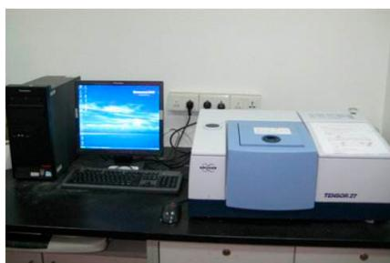
**Figure 5.** FTIR spectrometer.
