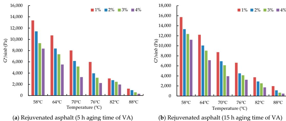
Figure 16. Influences of WCO on rutting resistance factor of rejuvenated asphalt (different aging time of VA).
