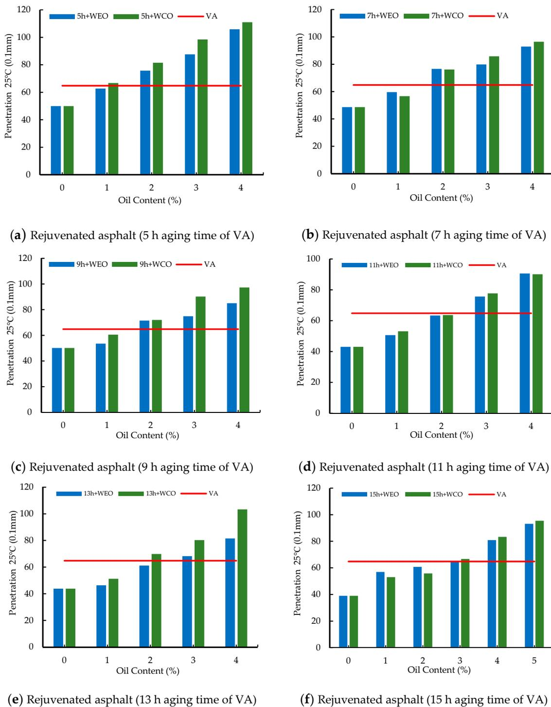
Figure 6. Effects of WEO or WCO on penetration of different aged asphalt.
