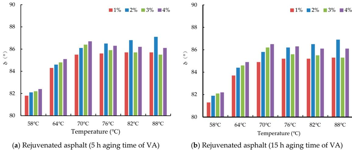
Figure 11. Influences of WEO on phase angle of rejuvenated asphalt (different aging time of VA).
