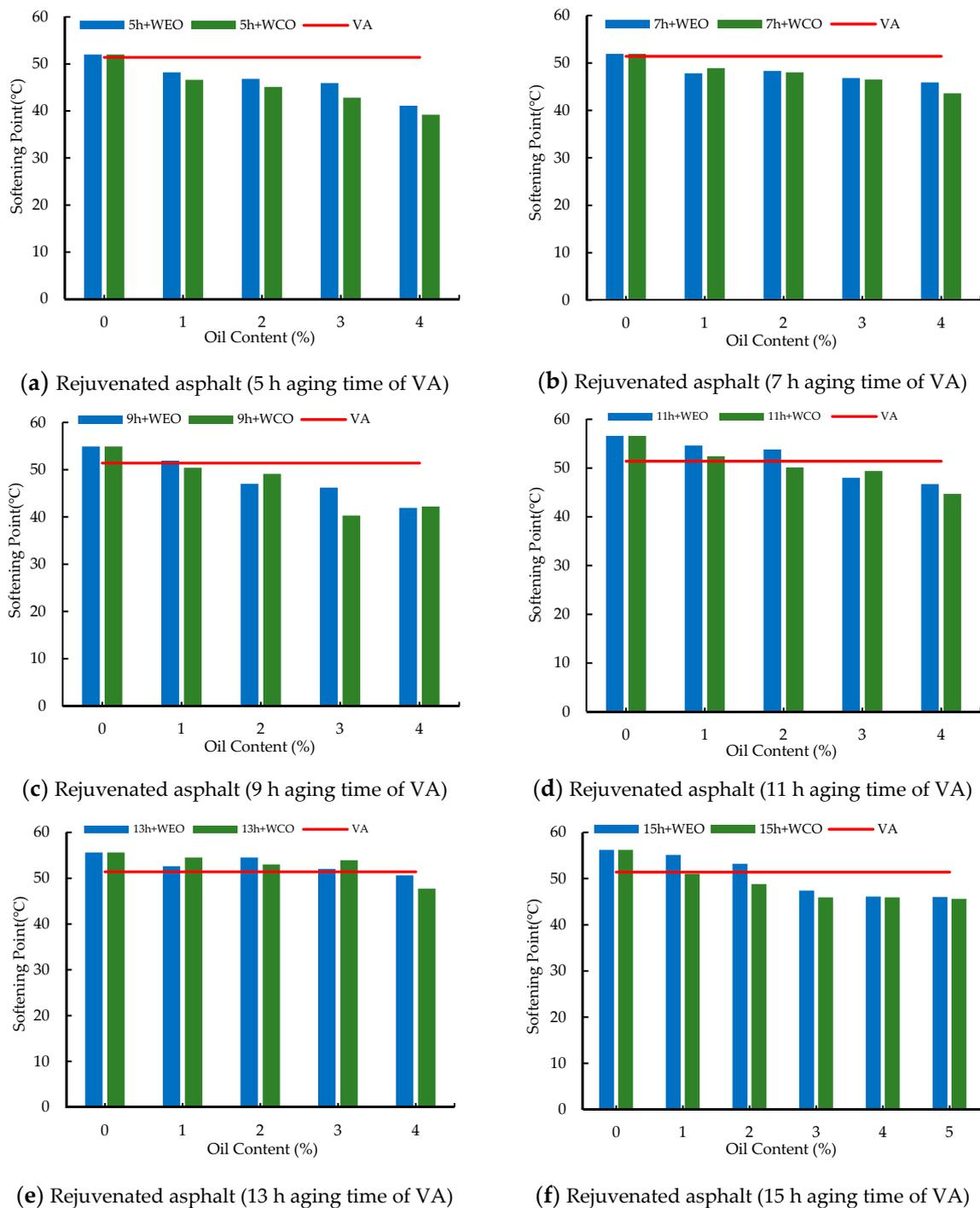
Figure 7. Effects of WEO and WCO on softening point of different aged asphalt.
