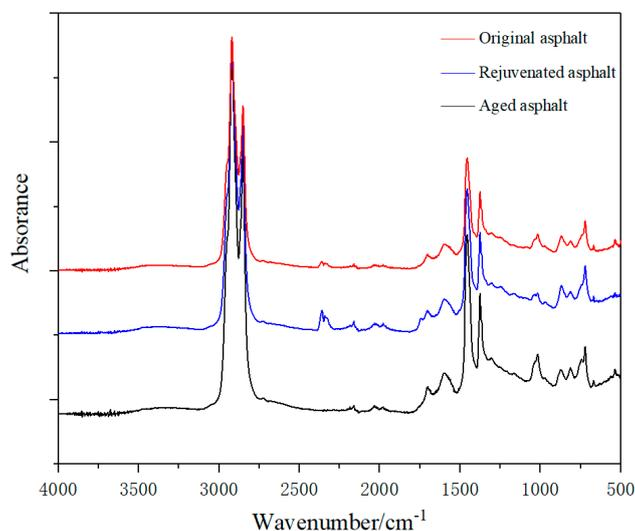
**Figure 10.** FTIR spectra results of VA, aged asphalt, and rejuvenated asphalt.
