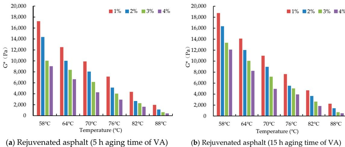
Figure 14. Effects of WCO on complex modulus of rejuvenated asphalt (different aging time of VA).
