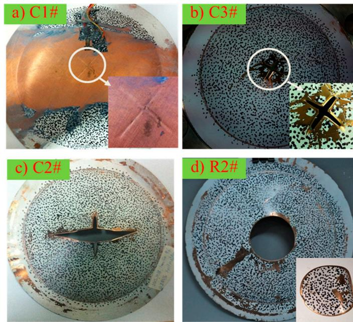
**Figure 17.** Failure modes of copper plates with pre-notches: (a) large ductile deformation and local necking (mode Ic failure); (b) splitting (mode II failure); (c) splitting and tearing (mode IIc failure); (d) fragment (mode III failure).
