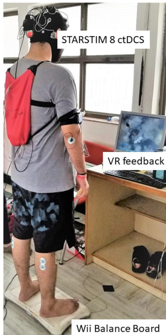
**Figure 1.** Portable experimental setup for the clinical study consisting of the Wii Balance Board to measure the center of pressure (CoP), a small form factor desktop PC with monitor for the virtual reality (VR) balance testing and training based on CoP. And the wireless STARSTIM 8 simulator for cerebellar transcranial direct current stimulation (ctDCS).
