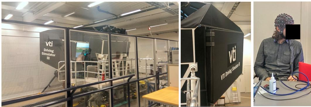
**Figure 1.** VTI simulator III and electroencephalography (EEG) electrodes setup on a participant.
