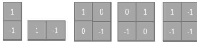
**Figure 1.** The architecture of the predefined filters.
