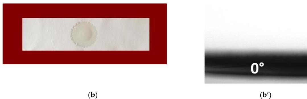
**Figure 3.** Images of distilled water droplets deposited on the surface of mats: (a) and (a'). CA; (b) and (b'). CA/PEG/QUE.
