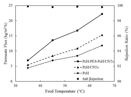
Figure 9. Permeate flux vs. feed water temperature for different membranes.
