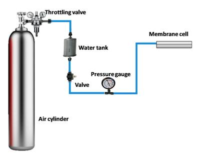
Figure 2. The liquid entry pressure investigation set up.
