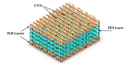
**Figure 1.** Schematic of the prepared triple-layer nanocomposite membrane.
