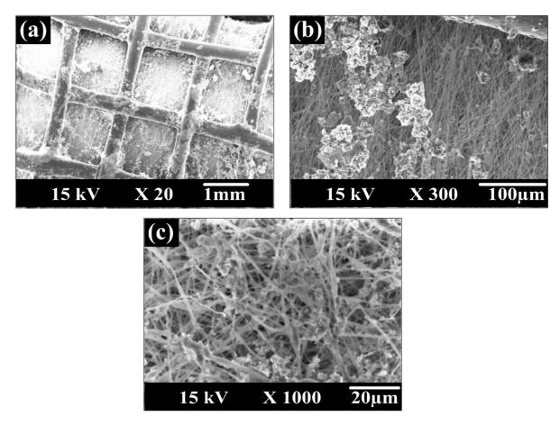
Figure 12. SEM images of the formed scales on (a) the spacer, (b) and (c) PcH-PES-PcH/CNTs nanocomposite membrane fibers, and with higher magnifications.
