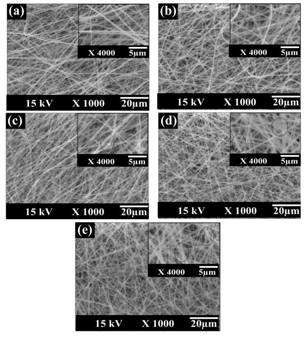
**Figure 6.** SEM images for the prepared membranes surface: (a) pure polyethersulfone (PES), (b) PES/carbon nanotubes (CNTs), (c) Pure poly (vinylidene fluoride-co-hexafluoro propylene (PcH), (d) PcH/CNTs, and (e) triple-layer PcH-PES-PcH/CNTs nanocomposite membranes.
