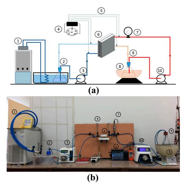
**Figure 4.** (a) Schematic diagram and (b) Photo of the used experimental test setup: 1. Thermostatic bath equipped with circulator, 2. Permeate flask, 3. Permeate pump, 4. Data logger, 5. Thermocouples, 6. MD Cell, 7. Pressure meter, 8. Heating bath, 9. Feed flask, and 10. Feed pump.
