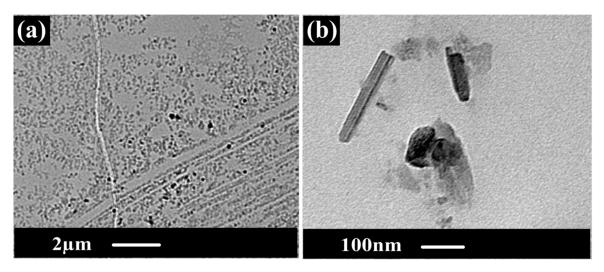
**Figure 7.** TEM cross-section images for the PcH-PES-PcH/CNTs membrane at different scales. (**a**) shows the homogenous distribution of CNTs; (**b**) the average size of CNTs.
