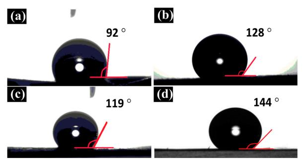
**Figure 8.** Contact angle results for (**a**) pure PES, (**b**) pure PcH, (**c**) PES/CNTs, and (**d**) PcH-PES-PcH/CNTs, which is almost the same as PcH/CNTs.
