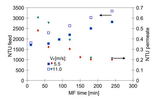
**Figure 8.** Changes in feed and permeate turbidity during MF of 1,3-PD fermentation broth with *Citrobacter freundii*. Module M4, TMP = 0.08 MPa.
