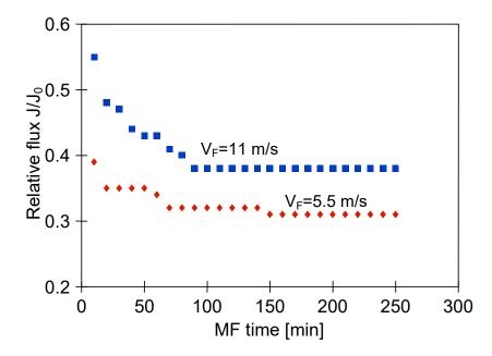
**Figure 7.** Effect of feed flow velocity on the relative permeate flux during MF of 1,3-PD fermentation broth with *Citrobacter freundii*. Module M4, TMP = 0.08 MPa,  $J_0 = 311 \text{ l/m}^2\text{h}$ .
