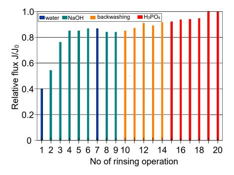
**Figure 12.** The efficiency of cleaning the ceramic membrane after the MF of 1,3-PD fermentation broth with *Citrobacter freundii* ( $V_F = 5.5 \text{ m/s}$ . TMP = 0.08 MPa). Operation time: water—30 min, NaOH—5 min, backwash—5 min, acid—10 min.
