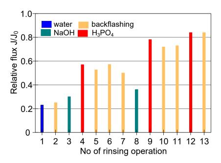
**Figure 16.** The efficiency of cleaning the ceramic membrane after the MF (TMP = 0.08 MPa,  $V_F = 5.5 \text{ m/s}$ ) of 1,3-PD fermentation broth with *Lactobacillus casei*. Operation time: water—30 min, backwash—5 min, NaOH—60 min, acid—60 min.
