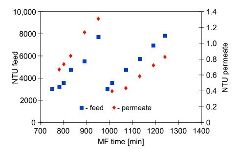
**Figure 10.** Changes in feed and permeate turbidity during the last two measurement series of the MF of 1,3-PD fermentation broth with *Citrobacter freundii*. Module M1, TMP = 0.03 MPa,  $V_F = 0.8 \text{ m/s}$ .
