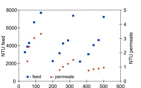
**Figure 5.** Changes in feed and permeate turbidity during MF of 1,3-PD fermentation broth with *Citrobacter freundii*. Module M1, TMP = 0.03 MPa, V<sub>F</sub> = 0.8 m/s.
