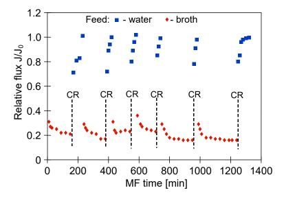
**Figure 9.** Changes in relative permeate flux during the long-term MF process of 1,3-PD fermentation broth with *Citrobacter freundii*, with periodically cleaning the module with 1% sodium hydroxide (NaOH) solution. Module M1, TMP = 0.03 MPa,  $V_F = 0.8 \text{ m/s}$ , CR—chemical cleaning.
