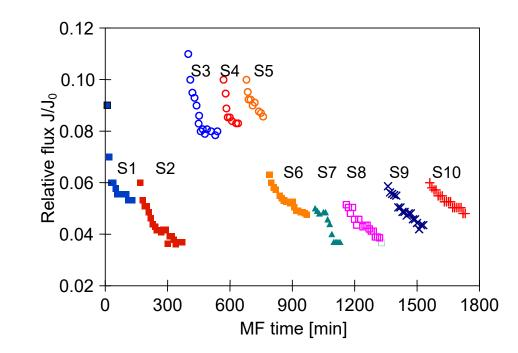
Figure 18. Changes in relative permeate flux during the long-term MF process of yeast suspension. Module M3, TMP = 0.08 MPa,  $V_F = 5.5$  m/s.
