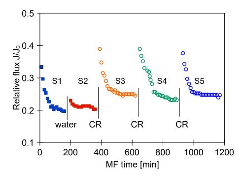
**Figure 15.** Changes in relative permeate flux during the long-term MF process of 1,3-PD fermentation broth with *Lactobacillus casei* with periodically cleaning the module. Module M4, TMP = 0.08 MPa,  $V_F = 5.5 \text{ m/s}$ , CR—chemical cleaning.
