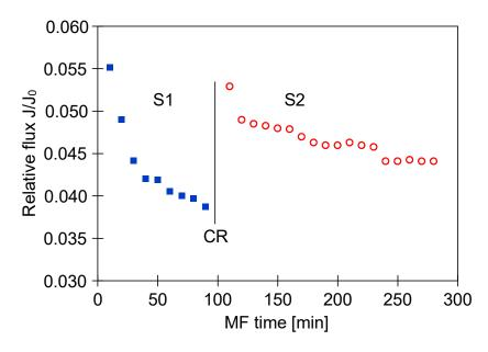
**Figure 22.** Changes in relative permeate flux during the MF process of yeast suspension with periodically cleaning the module. Module M4, TMP = 0.08 MPa,  $V_F = 5.5$  m/s, CR—chemical cleaning.
