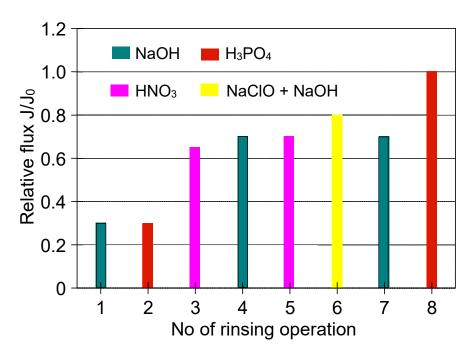
**Figure 24.** The efficiency of cleaning the ceramic membrane after the MF of yeast suspension (the second series of measurements). Operation time: 2% NaOH—60 min, 1% H<sub>3</sub>PO<sub>4</sub>—30 min, 2% HNO<sub>3</sub>—30 min, 2 L of 1% NaOH + 200 mL NaClO—60 min.
