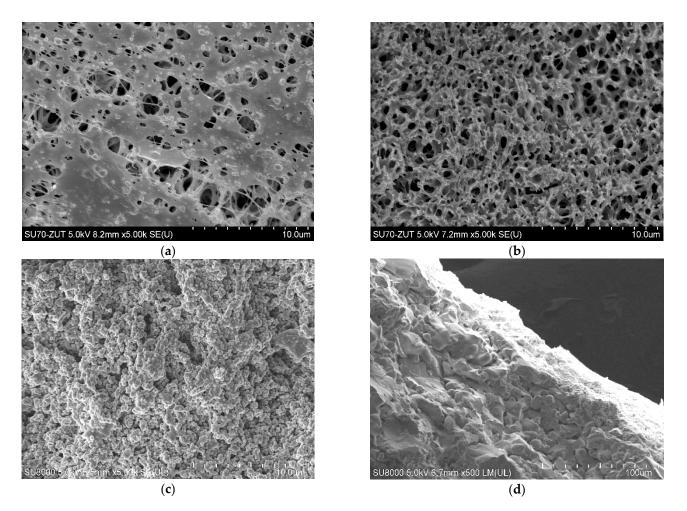
Figure 2. SEM images of tested membranes. Accurel PP S6/2 membrane: (a) surface, (b) cross-section, ceramic membrane: (c) surface and (d) cross-section.
