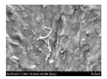
**Figure 6.** SEM image of PP S6/2 membrane (module M1) surface covered by deposit after MF process of fermentation broth with *Citrobacter freundii*. Deposit formed during 6 h of MF process.
