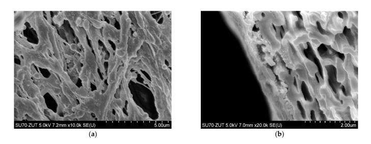
**Figure 21.** SEM images of PP membranes after cyclic chemical rinsing. (**a**) membrane surface, (**b**) membrane cross-section with deposit inside surface pores.
