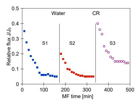
**Figure 17.** Changes in relative permeate flux during the long-term MF process of 1,3-PD fermentation broth with *Lactobacillus casei* with periodically cleaning the module. Module M2, TMP = 0.05 MPa,  $V_F = 1.5 \text{ m/s}$ , CR—chemical cleaning (NaOH).
