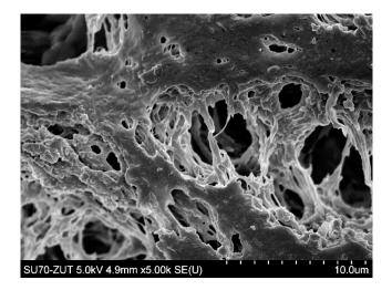
**Figure 11.** SEM image surface of Accurel PP S6/2 membrane. Module M1—membranes several times rinsed with 1% NaOH solution.
