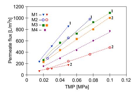
**Figure 3.** The maximum permeate flux as a function of transmembrane pressure (TMP): 1—after one operation of membrane wetting, 2—stabilized  $J_0$  values after several operations of membrane wetting.
