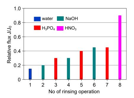
**Figure 23.** The efficiency of cleaning the ceramic membrane after the MF of yeast suspension (the first series of measurements). Operation time: water—30 min, 2% NaOH—40 min, 1% H<sub>3</sub>PO<sub>4</sub>—40 min, 2% HNO<sub>3</sub>—30 min.
