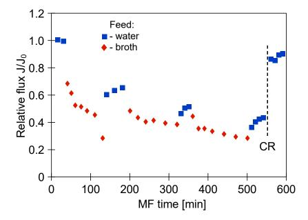
**Figure 4.** Changes in relative permeate flux during microfiltration (MF) of 1,3-propanediol (1,3-PD) fermentation broth with *Citrobacter freundii*. Module M1, TMP = 0.03 MPa,  $V_F = 0.8$  m/s, CR—chemical cleaning (1% NaOH).
