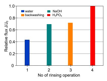
**Figure 13.** The efficiency of cleaning the ceramic membrane after the MF of 1,3-PD fermentation broth with *Citrobacter freundii* ( $V_F = 11 \text{ m/s}$ . TMP = 0.08 MPa). Operation time: water—30 min, NaOH—25 min, backwash—25 min, acid—50 min.
