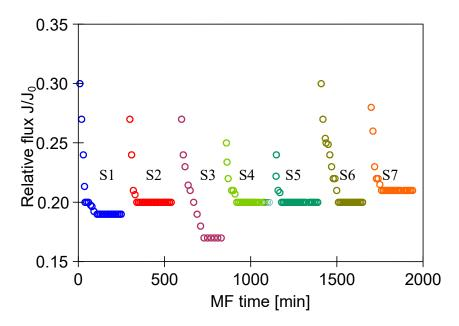
**Figure 14.** Changes in relative permeate flux during the long-term MF process of 1,3-PD fermentation broth with *Citrobacter freundii*. Module M4, TMP = 0.02 MPa, V<sub>F</sub> = 5.5 m/s, CR—chemical cleaning.
