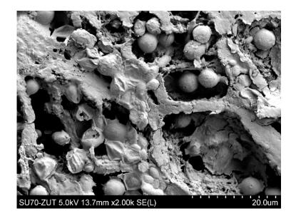
**Figure 19.** SEM image of PP S6/2 membrane (module M3) surface covered by biological deposit with yeast cells after MF process of yeast suspensions.
