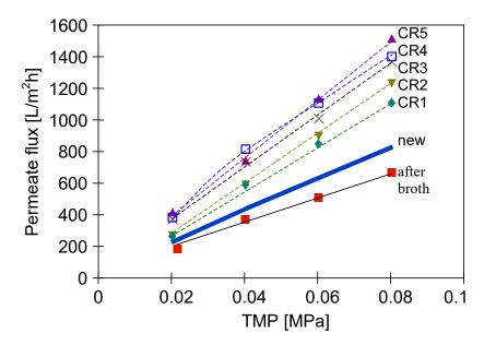
**Figure 20.** Effect of chemical membrane cleaning on the maximum permeate flux. Module M3. CR—chemical rinsing.
